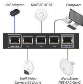
Example of a CPE Deployment for the ER-X
