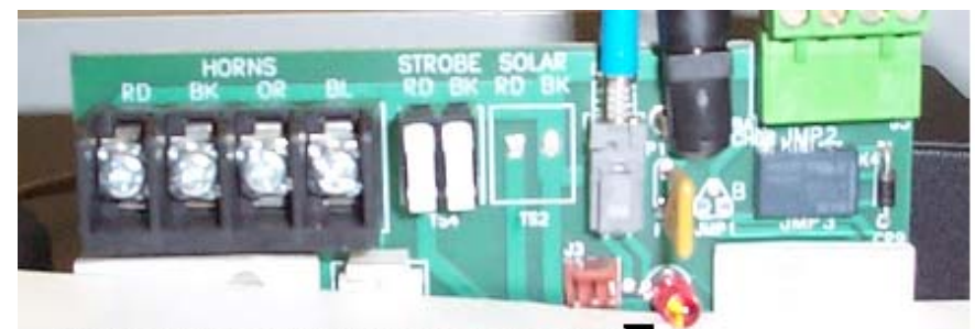
Battery Charging Indicator →
